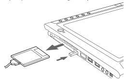
Figure 2-4 Removing a PC Card
